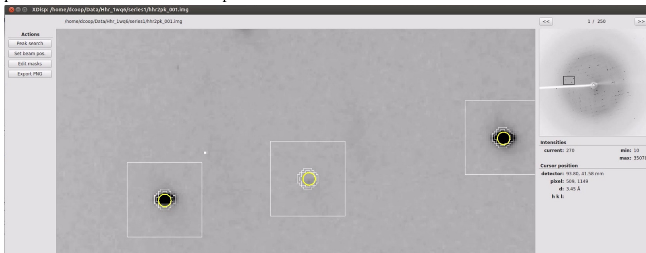
Figure 12. Integration boxes can be displayed to show what is considered the peak, background, and guard region.
